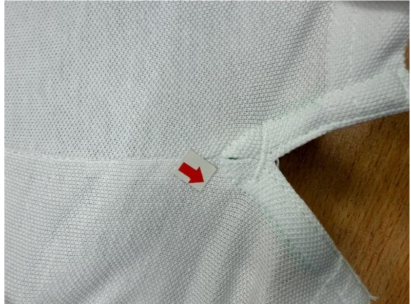
Open seam at side slit view
